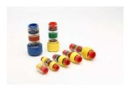
An active gas block connector has an internal seal that can be open to permit blowing through, or closed so the seal contacts the fibre and prevents the flow of gas.
